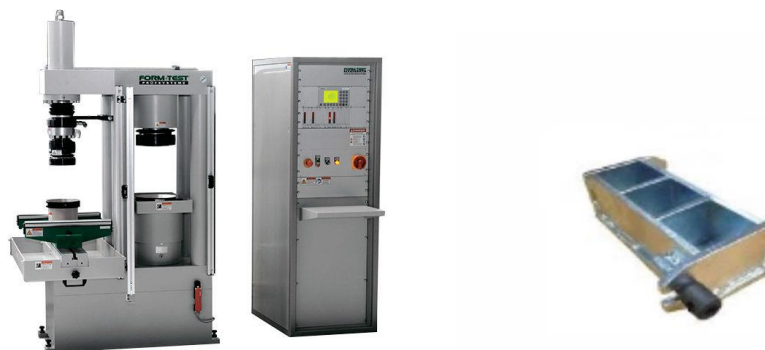
Figure 3 – Hydraulic press and forms for strength determination
