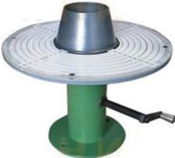
Figure 2 – Apparatus for shaking and compacting the mixture in the cone
